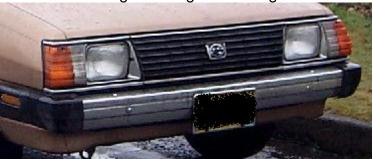
83-87 GL had quad headlight set-up with turn signals in the bumper
